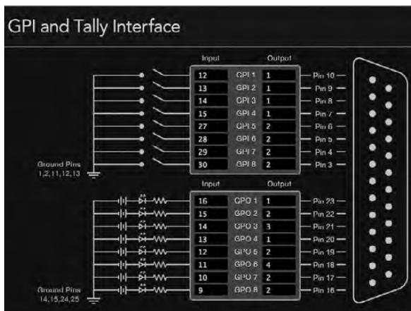
Click inside the diagram to change inputs and outputs for GPI crosspoint switching and Tally.
