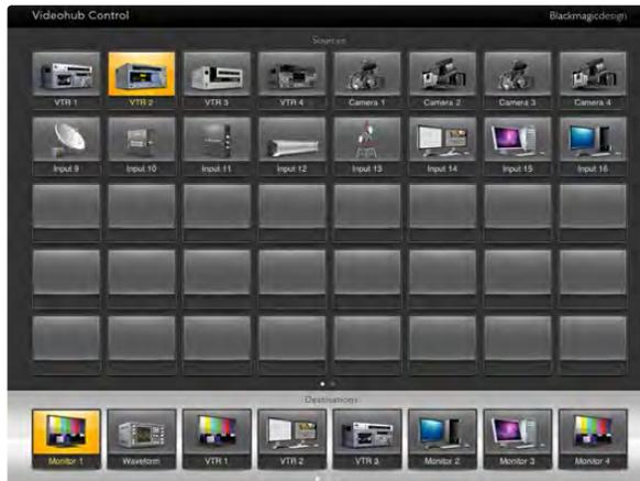
In order to see which video source has been routed to a video destination, tap a destination button and the associated video source button will illuminate.
