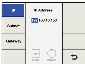
Press the MENU button to enter the network configuration page and use the TAKE button and the rotary knob to set the fields of the IP address.
