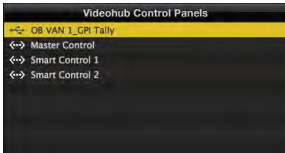
GPI and Tally Interface connected via USB
