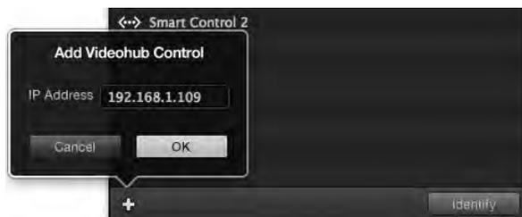
You can manually add a Videohub control panel, by IP address, to the list of Videohub Control Panels
