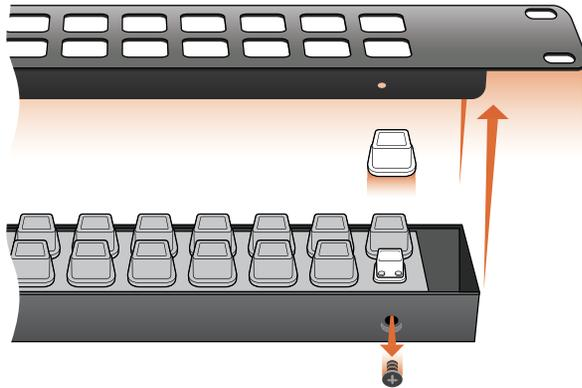
For Videohub Smart Control and Smart Videohub, remove the 8 screws, lift off the face plate and then the button caps.
