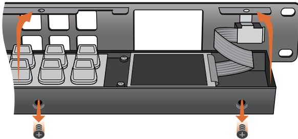
For Videohub Master Control, remove the 8 screws, lift off the face plate and carefully allow the face plate to lie down next to the rest of the unit. Then remove the button caps.
