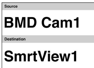
The LCD provides instant feedback of route selections and changes and allows you preview source and destination video without an external monitor.
