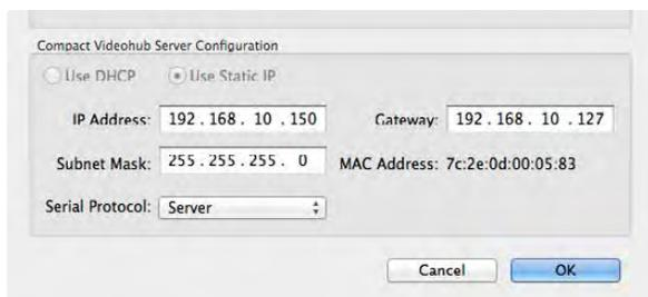
The Videohub Server Configuration options will only become active when an Ethernet-equipped Videohub is connected via USB.
