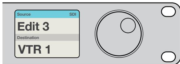
If you know that you want Edit 3 as the source, and VTR 1 as the destination, you can select the route directly without any scrolling being necessary. In this example, press DEST, press the customized VTR button and then press 1. VTR 1 will be shown in the destination field. Now press SRC, press the customized Edit button and then press 3. "Edit 3" will be shown in the source field. Finally, press TAKE to confirm the route change.
