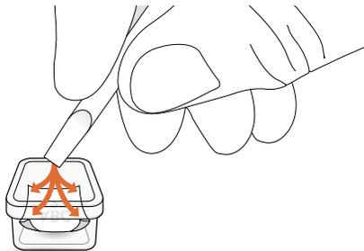
Lightly press the four corners of the square label into the rounded corners of the clear cap
