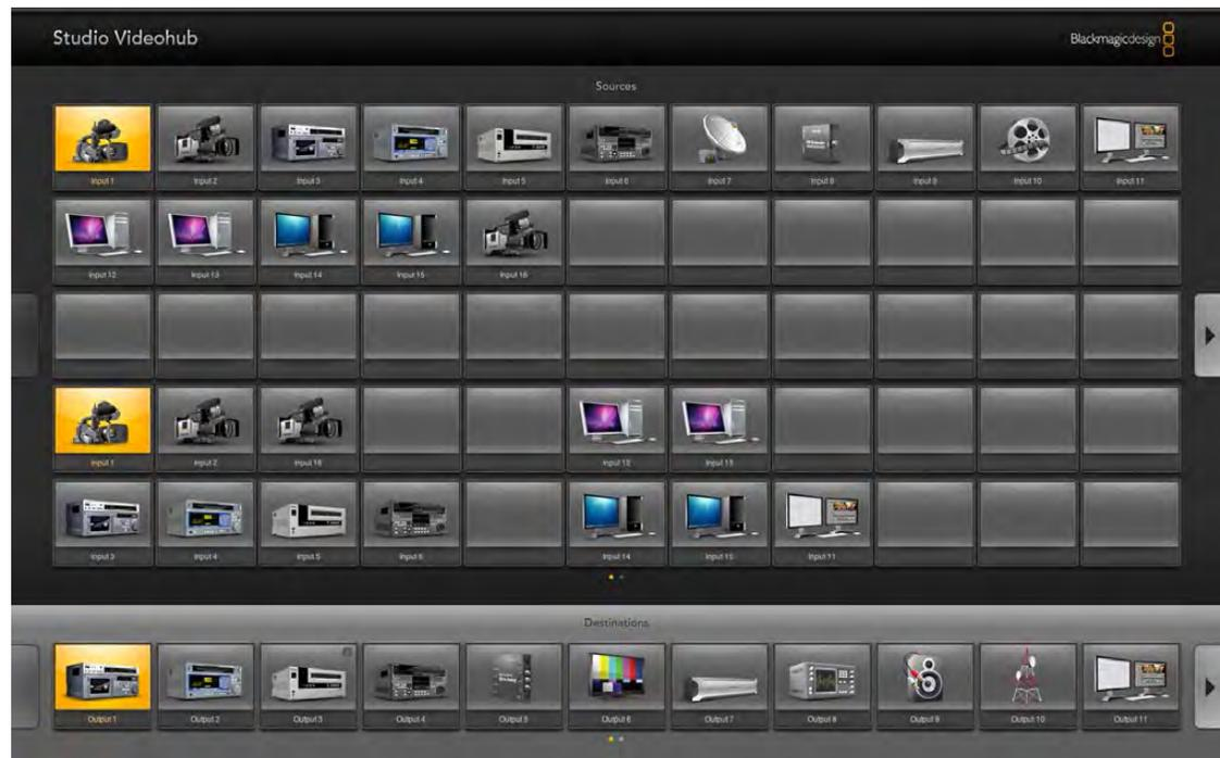
Full Screen 24" Pushbutton view showing an example of duplication and grouping of inputs. Two, illuminated instances of Input 1 can be seen in this example. Grouping of inputs can enable quick identification and location of video sources of the same type, e.g. all available cameras.
