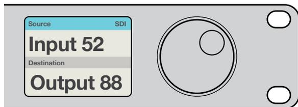
If you've chosen to keep the default labels for all Videohub SDI and remote ports, you can simply type the port numbers to make a routing change. In this example, press DEST and then type the port number 88. Then press SRC and type the port number 52. Press TAKE to confirm the route change.
