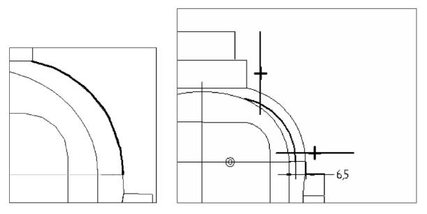
Type an offset distance of 6.5 mm and press ENTER.
