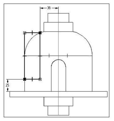
On the Draw toolbar, click the Select Tool. Select the profile by clicking to the top and left of the profile, holding, and dragging to the bottom and right of the profile.
