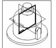
Draw the profile shown. Notice the connect relationships between the top right and bottom left corners of the rectangle and the outer line of the revolved protrusion.
